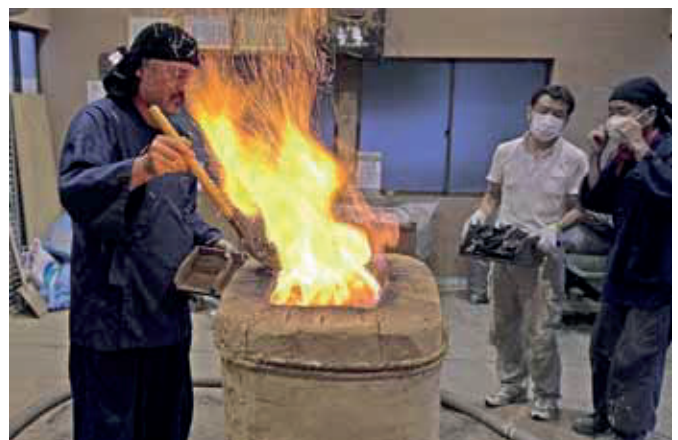
First charging of the ore in the Tataru furnace
