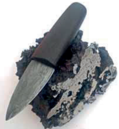
Bloom and knife from the 2018 "God Furnace" by Robert Seiler (see cover) Photo James Wood
