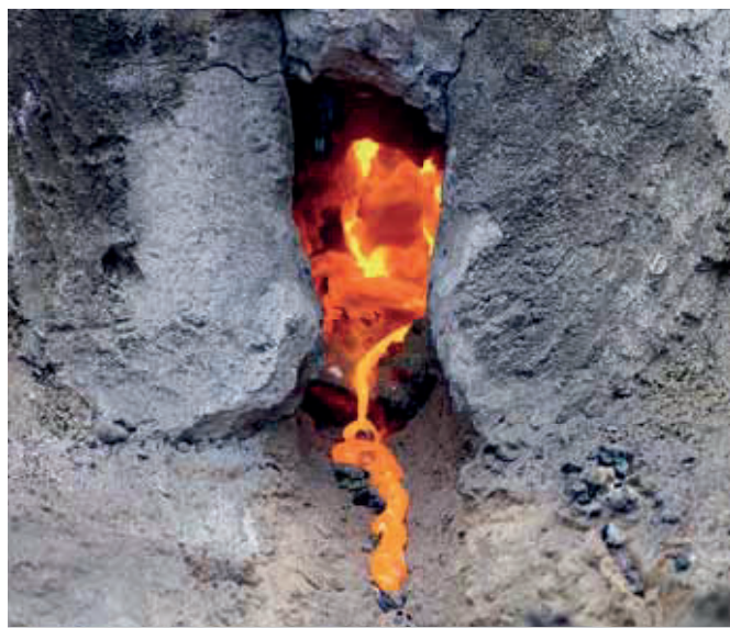
Tapping slag during the smelt
